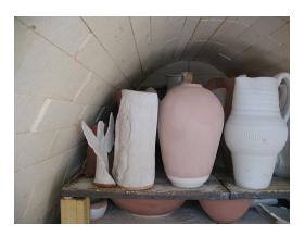
These clay pots have been dried and they have just been loaded into a kiln to be fired. <sup>8</sup>
