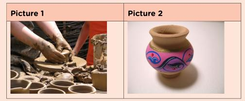
In Picture 1 the clay is wet and soft. It has been mixed with some water so it can be moulded. In Picture 2 the clay is hard and dry. But it is also brittle as if you drop it on the floor it will smash. To get from the clay in Picture 1 to the pot in Picture 2, the clay was moulded into a specific shape and then left to
