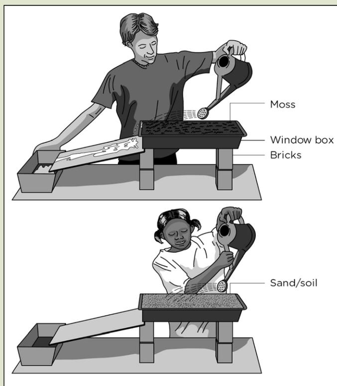
*Setup for the drainage experiment.*
