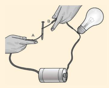
Test each object as shown here with the nail.
