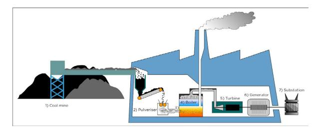
The process of making electricity from coal in a power station.
