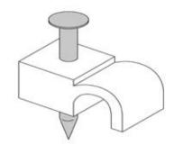
A clip to hold telephone cables to the wall.
