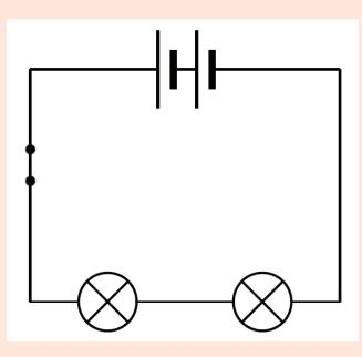
Two cells, two bulbs, a switch and 4 connecting electric wires.
