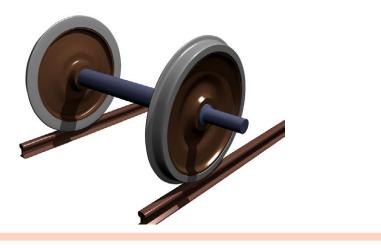
You know there are different ways to let wheels turn on an axle. One way is to have the axle fixed to the body, and the wheels are free to turn on the axle. What is the other way to let wheels turn?
