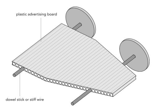
The board makes bearings for the axles which are fixed to the wheels. The axles turn in the holes.
