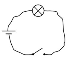
BUT for electric circuit diagrams we represent the wires with straight lines.
