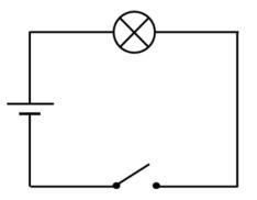
This is a simple and quick way to represent an electric circuit and it should be clear to everyone that this circuit has a battery, a bulb and a switch, all connected with electric wires. Although we draw the wires as straight lines in a circuit diagram, REMEMBER that in real life, the wires are not straight. Just think of the electric wires that are attached to the appliances in your home, like to a kettle, a lamp, a vacuum cleaner or a computer.
