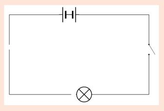
batteries: one battery pushes current one way, the other the other way, so no current
