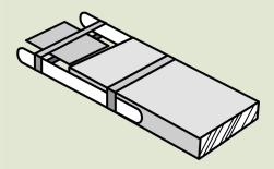
4. Turn the plastic to twist the rubber band.
