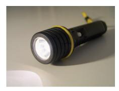
Chemical energy in the battery in the torch is changed into electrical energy which is changed into light.
